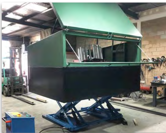
Manufacture of trap to housing showing hydraulics enabling trap to be raised or lowered
