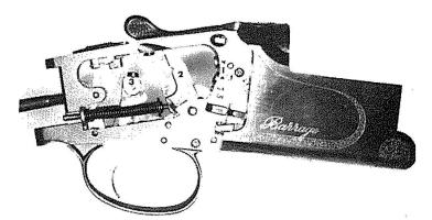
• The trigger assembly is very well designed. Here shown in the cocked situation. 1 are the firing pins, note the good angle of attack. 2 are the hammers, both cocked. 3 is the inertia block which on recoil will set the sear for the second barrel. The gun is not selective as is the norm in trap guns these days and so the trigger assembly is very uncluttered.
