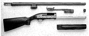
1. stock and action, 2. barrel, 3. breech bolt and cocking rod, 4. fore-end. Disassembly and assembly is simple and requires no tools.
