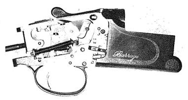
• The same thing with the bottom barrel fired. Note the coil springs for hammer power and the neat way the hammer fits the contour of the action when at rest.
