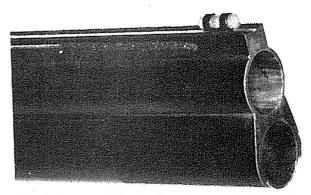
• The business end showing the unique way the bottom barrel is suspended at the muzzle.
