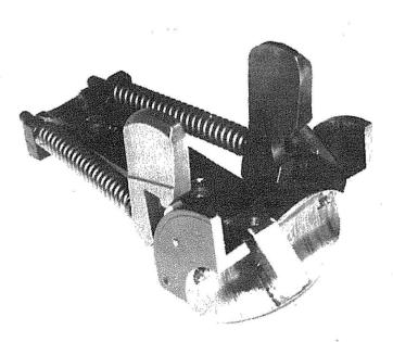
• Ejection mechanism in the forend iron. Note how big the ejection hammers are and the coil springs that power them. The cocking tang in the centre is easily replaceable.
