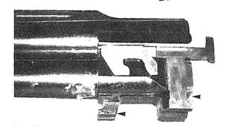
• The monobloc chamber assembly. Notice the hinge pin yoke and main lock up lump are grooved to allow the cocking rod to pass through. Ejector for the top barrel is out.
