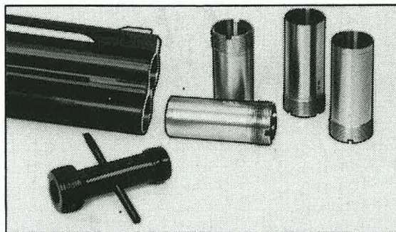
New flush mounting choke system that does not alter line of barrels. 4 chokes imp. cyl., mod., imp. mod., and full. Key/thread cleaner come with guns featuring the mobilchoke system.
