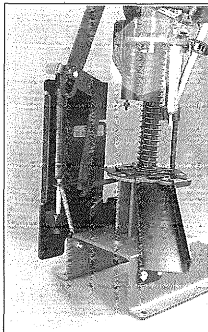
Energy from a gas strut is utilised to advance the "stage" of the press as each shell moves from station to station.
