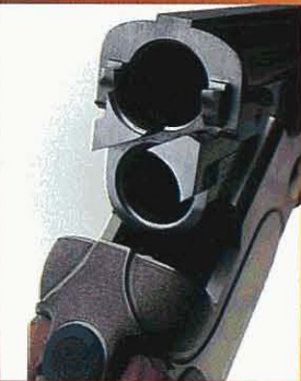
Traditional cross bolt locking system.
