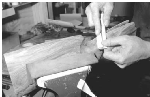
(Right) The finished shape of the stock is gently sanded to ensure flat and continuous lines.
