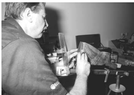
(Above) Locating the recoil pad, once the cast has been transferred to the stock is one of the initial steps.
