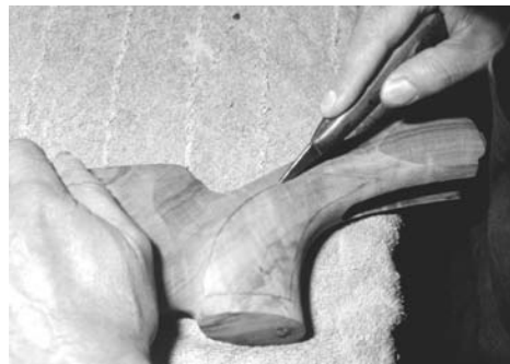
(Below) The first cuts with the checkering tool are to establish the border. The tool is moved gently and firmly to ensure continuity of the curve.
