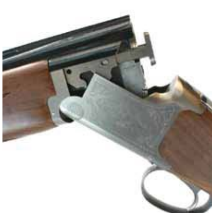
Browning has long used two-piece ejectors on its shotguns. These operated with precision timing on the review gun.
