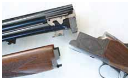
This take-down view of the gun shows the lug beneath the barrel, which couples with the pin across the front of the receiver. Also shown is the rearward lump, which fits into the bottom of the receiver, and its rearward trapezoid 'bite' that locks and secures the action.
