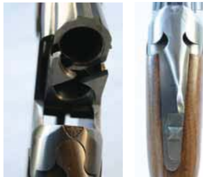
The rear of the barrel set, showing the split ejectors and highly polished receiver top. Browning has successfully used this rib design for years.
